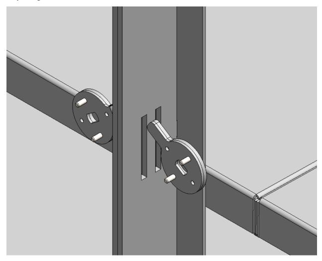
You can loosen the top two and the two bottom bolts for the center mullion and adjust the location by sliding back or front to fit the locks, then tighten again the bolts to secure the position of the center mullion.
