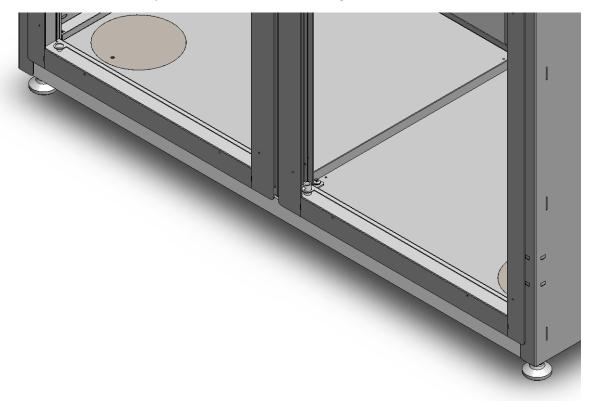
For the backs, you will just need to remove the circular plate on the inside, and adjust the footpad, then replace the circular plate.
