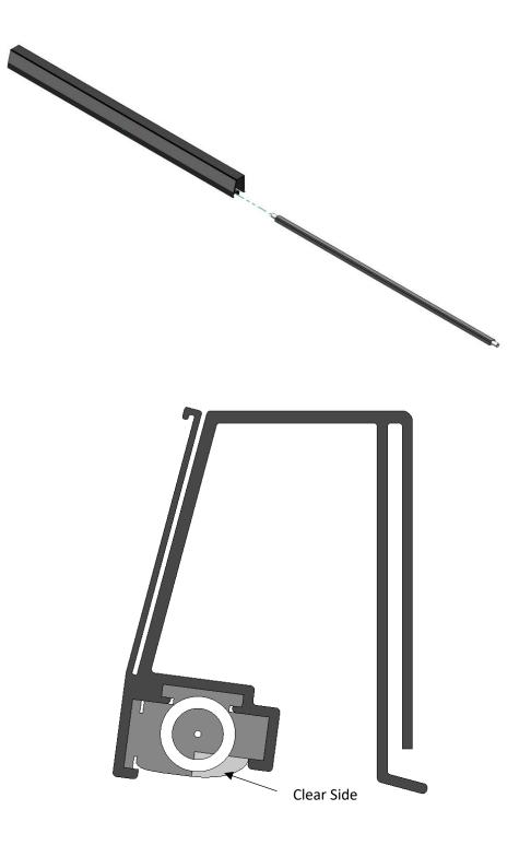
**Step3:** Insert the PTM with the led lights on the front of the shelves to bring light to the section below the shelf.
