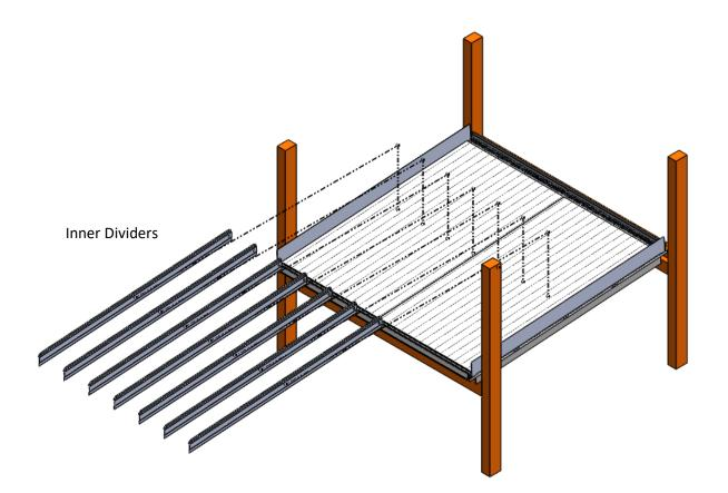
Dividers to be secure in the slots, folded side must be up and all indents must go the same way in each shelf
